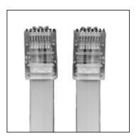
After crimping a RJ45 connector on one end of the eight wire cable, attach a connector on the other end "upside down" from the first so that when the connectors are placed side by side the wire orientation will appear as shown in the above illustration. <u>Check the cable with a continuity tester prior to installation.</u>
