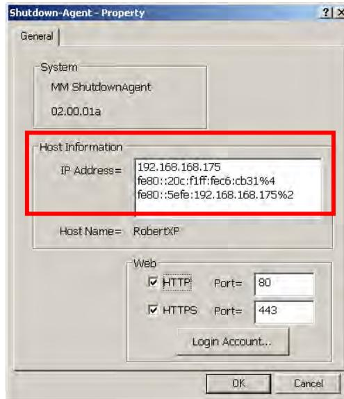
4. Go to SentryHD's SNMP Trap page and input the IP address of the MM ShutdownAgent's Host Server into the SNMP Trap table as the Target IP. Select the MM ShutdownAgent for the Event Level and UPSv4 as the Trap MIB.
