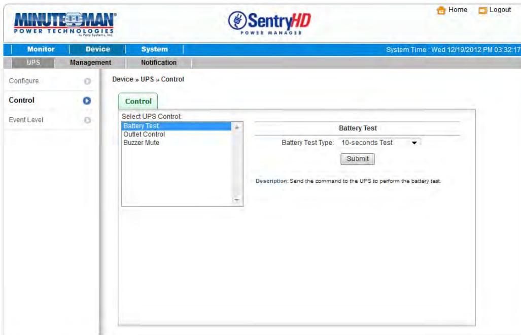
**Battery Test:** After you select the battery test type and click Submit SentryHD will send the command to the UPS to perform the selected battery test.
