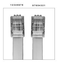
After crimping a RJ45 connector on one end of the eight wire cable, attach a connector on the other end with reversed orientation from the first so Pin 1 is on the opposite side of the cable from the first connector. <u>Check</u> the cable with a continuity tester prior to installation.
