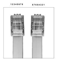
After crimping a RJ45 connector on one end of the eight wire cable, attach a connector on the other end with reversed orientation from the first so Pin 1 is on the opposite side of the cable from the first connector. Check the cable with a continuity tester prior to installation.
